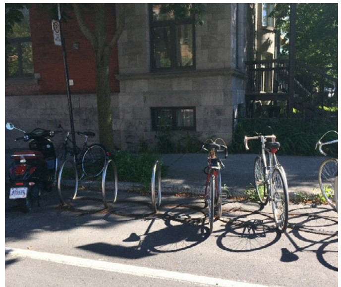
Figure 36: Two three-hoop bicycle racks, Montreal, QC; Credit: Julia Malmo-Laycock
