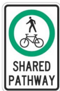
Figure 30: Shared-use path signage example; Credit: City of Edmonton
