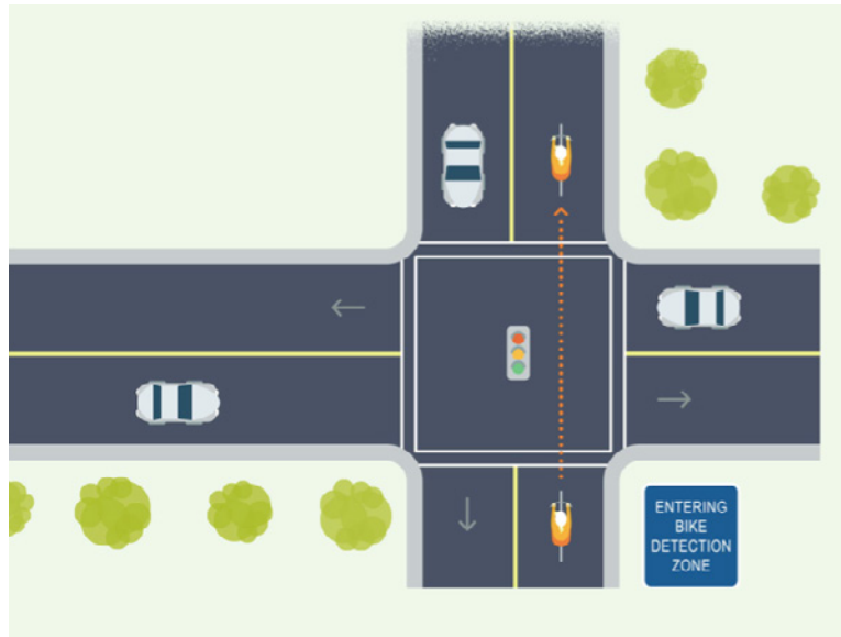
Figure 18: Bicycle detection intersection illustration; Credit: City of Edmonton Downtown Bike Network Education Booklet
