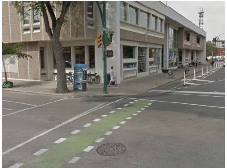
Figure 13: Painted bicycle lane through intersection, 23rd Avenue E and 4th Avenue, Saskatoon, SK. Credit: Google Maps
