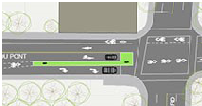
Figure 14: Bike box on Dupont Street, Quebec City, QC. Credit: Ville de Quebec
